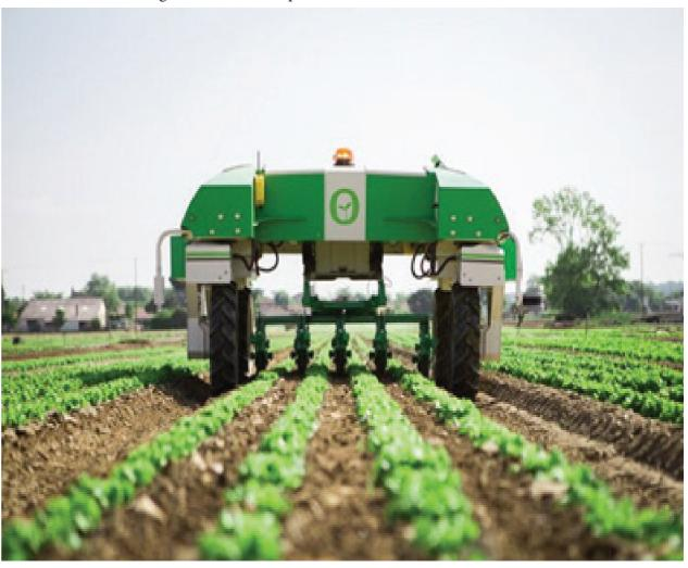
A popular example of agrobot is "Dino" - an agrobot developed in France that weeds crops. This robot is specific in mechanical weeding of vegetable crops; it identifies the weeds in the crop rows and can distinguish between the commercial plant and the weed with artificial intelligence (AI) applied to image recognition.
